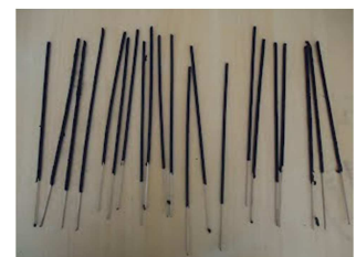
(f) Uniformly coated incense-stick with perfect circular cross-section is produced by the machine.
