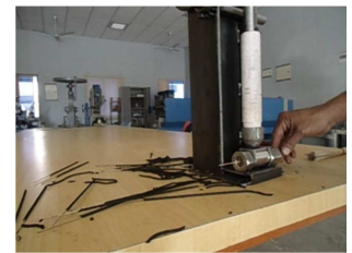
(b) Bamboo stick is fed until 20% of the stick is outside the die so that its uncoated
