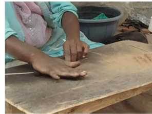
(c) A normal pressure is applied on the stick along with paste by the palm
