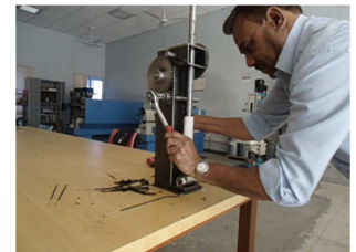
(d) The user rotates the handle by 30° such that stick is extruded out of die completely
