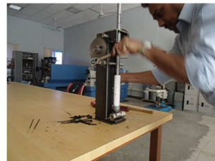
(c) The user starts cranking the handle; extrusion initiates
