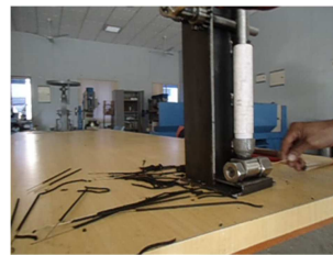
(a) The user is feeding the bamboo stick into the nozzle
