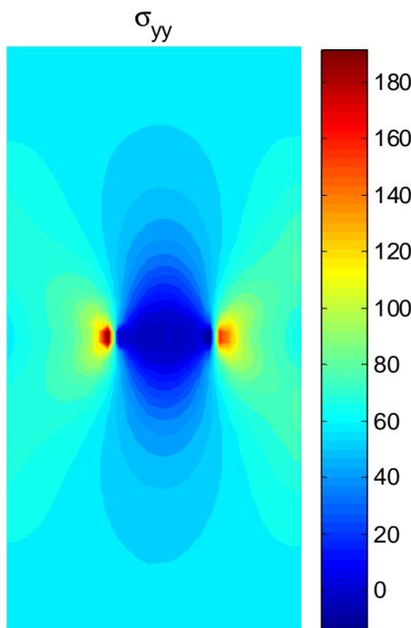
Fig. 6 Stress contour plot ( $\sigma_{yy}$ ) for centre crack in plate
