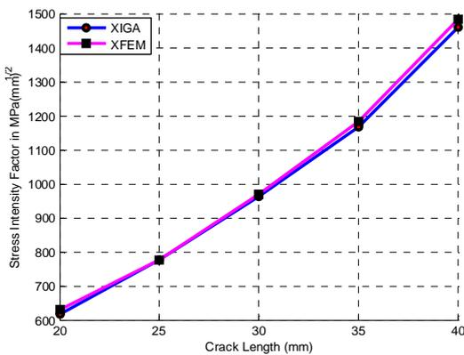
Fig. 11 SIF variation with crack length for double edge crack
