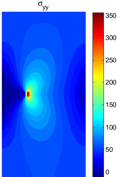
Fig. 2 Stress contour plot ( $\sigma_{yy}$ ) for an edge crack plate
