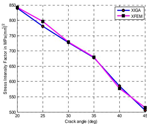
Fig. 12 SIF variation with crack angle for double edge crack
