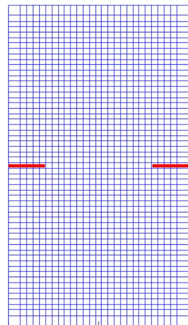
Fig. 9 Geometry of double edge crack in plate
