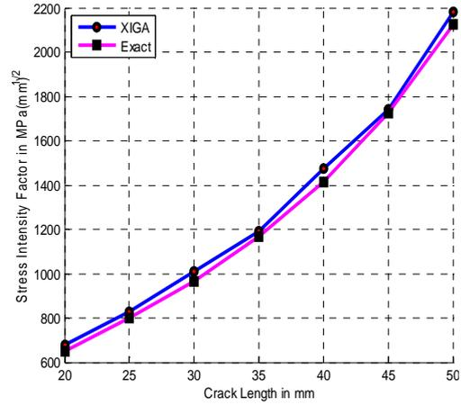
Fig. 3 SIF variation with crack length for a left edge crack problem
