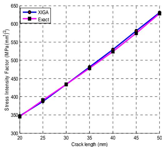
Fig. 7 SIF variation with crack length for centre crack
