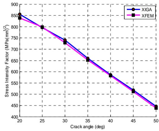
Fig. 4 SIF variation with crack angle for a left edge crack problem
