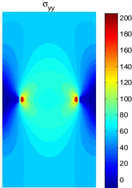
Fig. 10 Stress contour plot ( $\sigma_{yy}$ ) for double edge crack in plate
