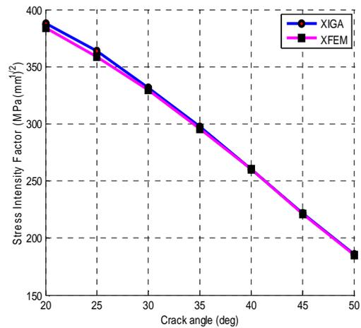
Fig. 8 SIF variation with crack angle for centre crack
