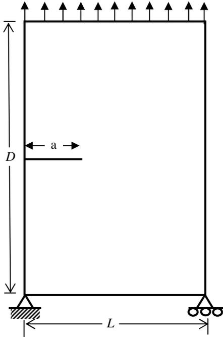
Fig. 1 Edge crack plate along with direction
