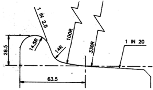
Fig. 6: Wheel Profile as per Indian railway standard
