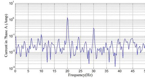
Fig. 9. Bridge current in Phase A at 20Hz supply frequency in frequency domain without mass in the disc
