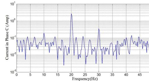
Fig. 11. Bridge current in Phase C at 20Hz supply frequency in frequency domain without mass in the disc
