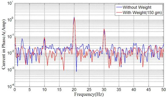
Fig. 15. Phase A current at 20Hz supply frequency with a mass of 150grams
