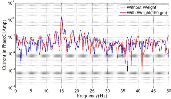
Fig. 14. Phase C current at 15Hz supply frequency with a mass of 150grams
