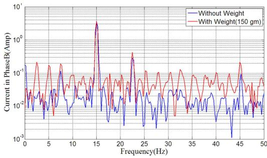
Fig. 13. Phase B current at 15Hz supply frequency with a mass of 150grams
