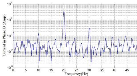
Fig. 10. Bridge current in Phase B at 20Hz supply frequency in frequency domain without mass in the disc
