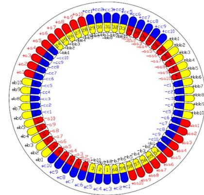
Fig. 2. A winding scheme of a distributed, double layered winding.
