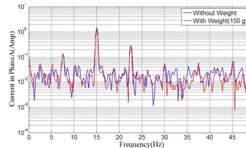
Fig. 12. Phase A current at 15Hz supply frequency with a mass of 150grams
