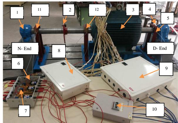
Fig. 1. A modified 37kW induction machine for the experimental setup.
