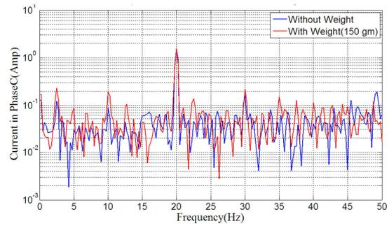
Fig. 17. Phase C current at 20Hz supply frequency with a mass of 150grams
