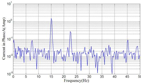
Fig. 6. Bridge current in Phase A at 15Hz supply frequency in frequency domain without mass in the disc
