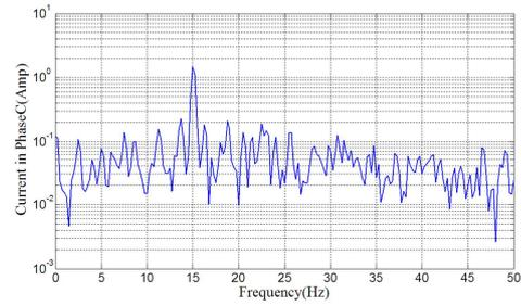
Fig. 8. Bridge current in Phase C at 15Hz supply frequency in frequency domain without mass in the disc
