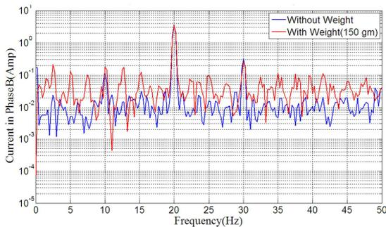
Fig. 16. Phase B current at 20Hz supply frequency with a mass of 150grams
