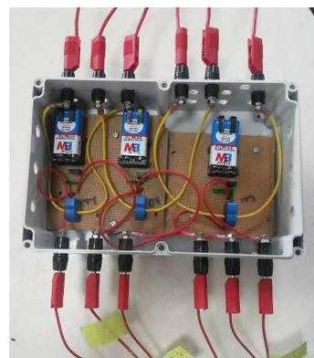
Fig. 5. A current transducer kit.
