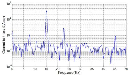
Fig. 7. Bridge current in Phase B at 15Hz supply frequency in frequency domain without mass in the disc
