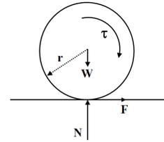
Fig. 5: Free body diagram of the wheel
