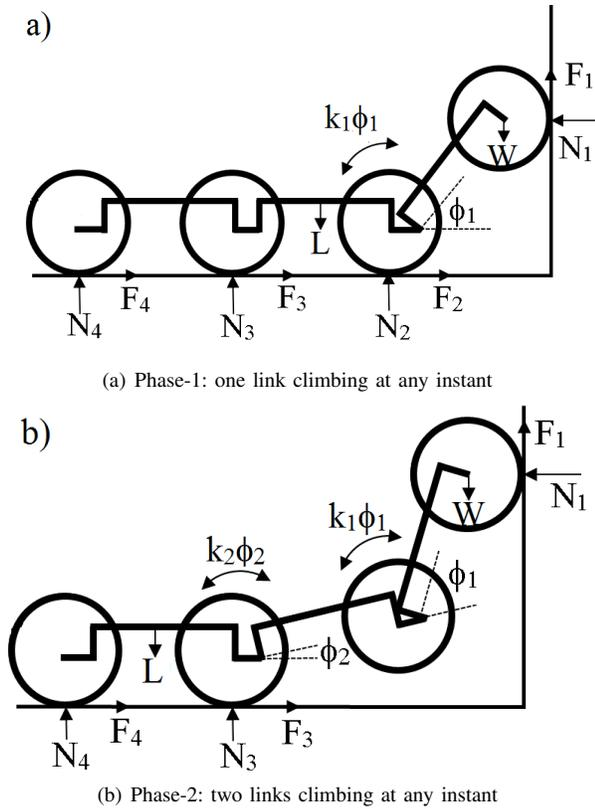
Fig. 4: Snapshots showing the various forces and moments acting on the robot during the 2 climbing phases
