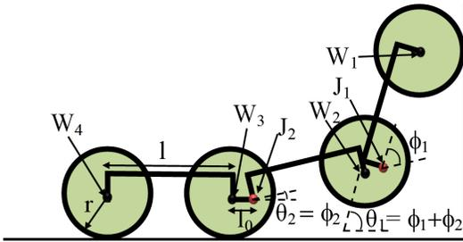
Fig. 2: Schematic of the 3-module robot
