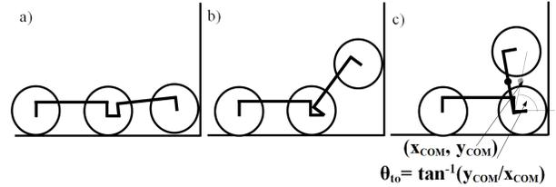
Fig. 3: A fully passive system failing to climb a big step like obstacle
