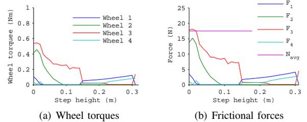
Fig. 7: Plots of optimized wheel torques and frictional forces against step height for all the 4 wheels
