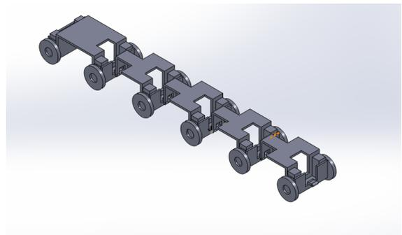
Fig. 1: CAD model of the proposed 3-module robot
