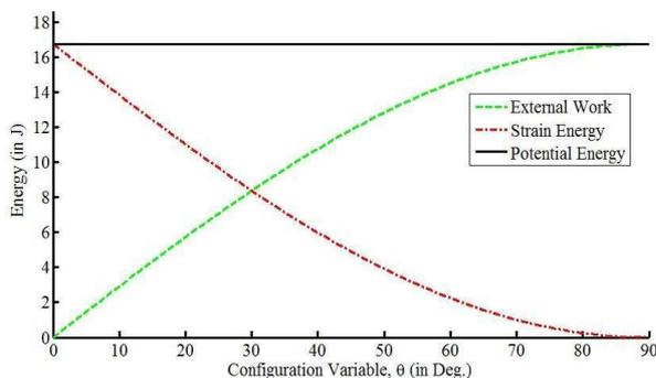
Fig. 13. Variation of the strain energy, external work, and potential energy for a statically balanced scissors mechanism.
