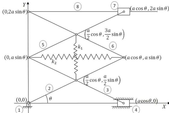
Fig. 11. Attaching two springs on the scissors mechanism for static balancing.
