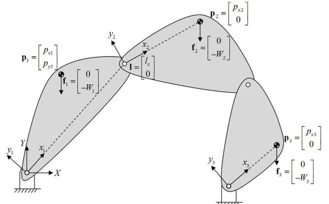
Fig. 6. Four-bar linkage under gravity loads.
