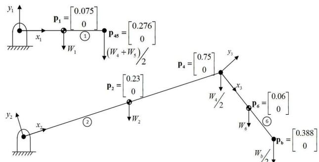
Fig. 10. Peaucellier-Lipkin linkage broken into two identical 2R linkages and a lever, which are balanced separately.
