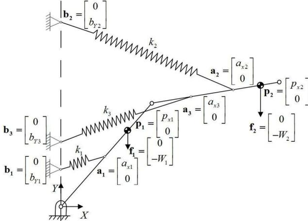
Fig. 4. Minimization of the potential energy of a simplified 2R linkage.
