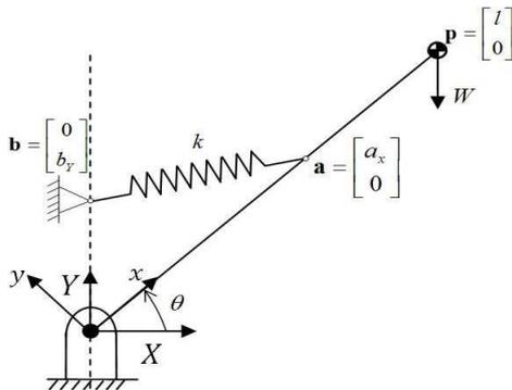
Fig. 1. Static balancing of lever under gravity load.
