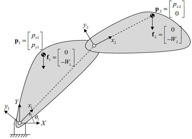
Fig. 5. General configuration of gravity loaded 2R linkage.
