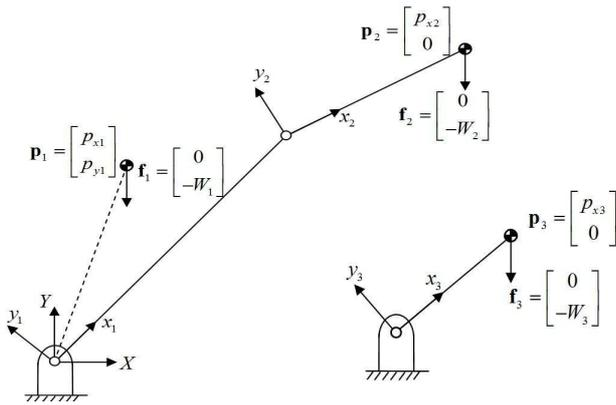
Fig. 7. Four-bar linkage broken into a 2R linkage and a lever, which are balanced separately.
