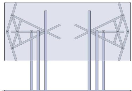
Fig. 9. Two identical Peaucellier-Lipkin linkages used for the vertical motion of a writing-board.
