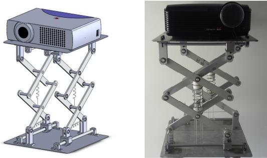
Fig. 12. Scissors mechanism used for the vertical motion of a projector.
