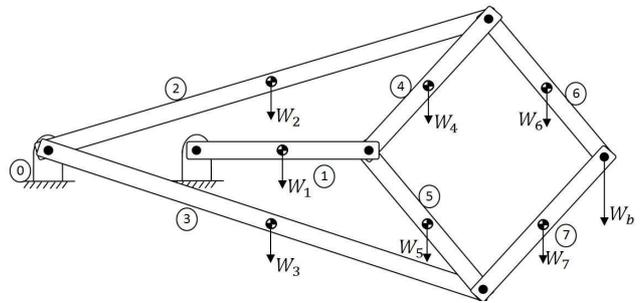
Fig. 8. Peaucellier-Lipkin linkage under gravity loads
