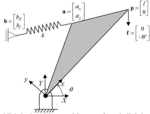
Fig. 3. Minimization of the potential energy of a statically balanced lever.
