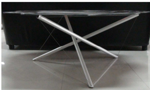
Fig. 4. Two views of the tensegrity table under the application of load. Free standing tensegrity table (blue lines indicate the bars and the red solid lines indicate the cables). The table under an applied external load (green dashed lines indicate the bars and the magenta dashed lines indicate the cables).
