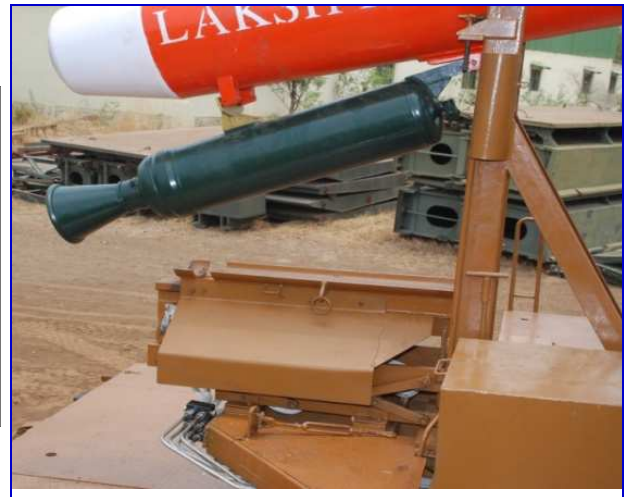
Fig.13 Realised Booster Mechanism (Closed condition)
