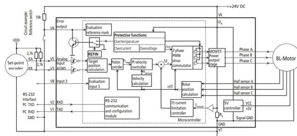
Figure 12: Circuit diagram of the controller. [17]
