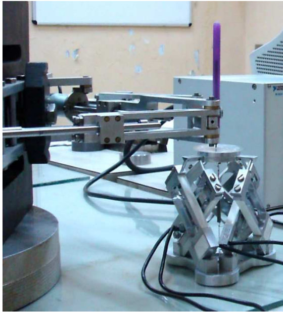
(a) Planar parallel Manipulator making an in-contact procedure with the environment fitted with a wrench sensor
