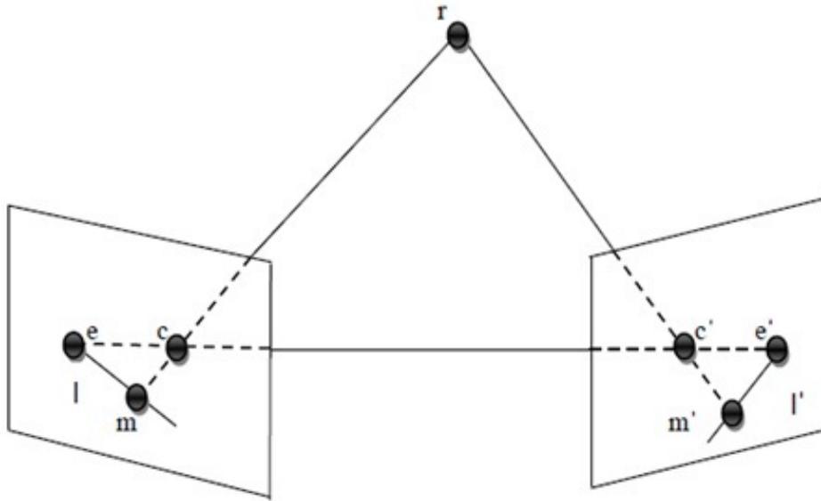
Fig. 1. The epipolar transformation.
