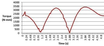
Fig. 13. Torque of upper actuator joint for 180 degree motion
