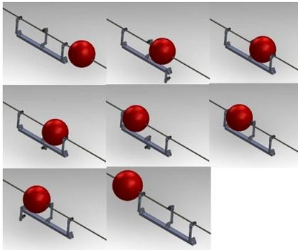
Fig. 10. CAD representations of obstacle avoidance manoeuvres
