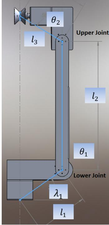
Fig. 12. Kinematics of arm
