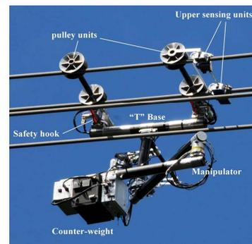
Fig. 2. Expliner Obstacle Avoidance [4]
