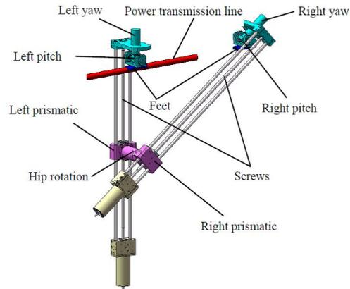
Fig. 5. Biped Line Walking Robot - CAD representation [21]
