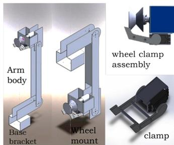
Fig. 8. CAD model of Arm, clamp, and wheel-clamp assembly
