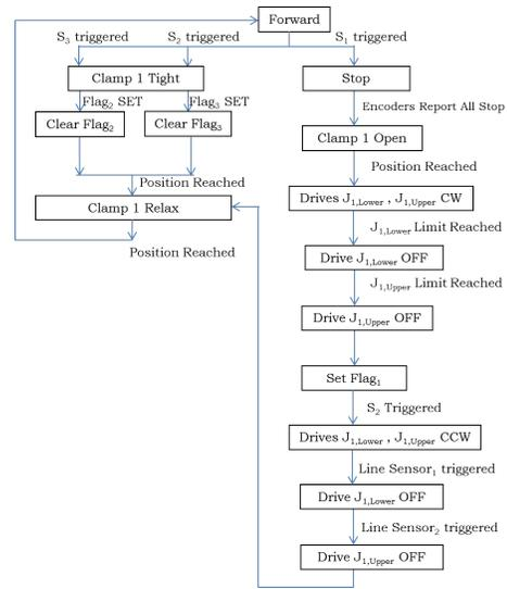
Fig. 11. State Machine for Obstacle Avoidance
