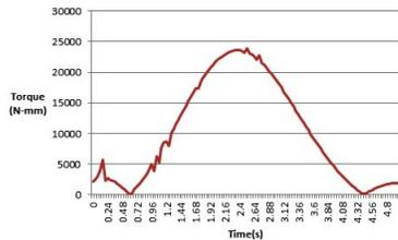
Fig. 14. Torque of lower actuator joint for 180 degree motion
