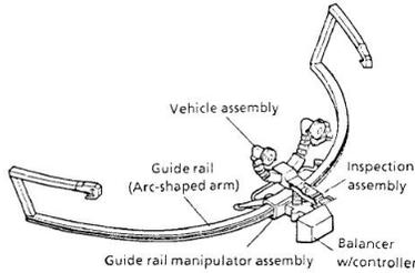
Fig. 3. Mobile robot for power line inspection [17]
