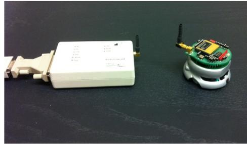
Fig. 2. Radio base and a radio turret mounted Khepera-II robot.
