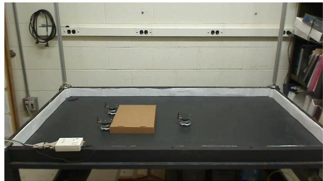
Fig. 7. The Khepera-II robots transporting a cardboard box across the arena.
