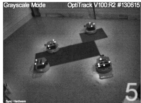
Fig. 1. Swarming robots carrying out a perimeter surveillance task. [29]
