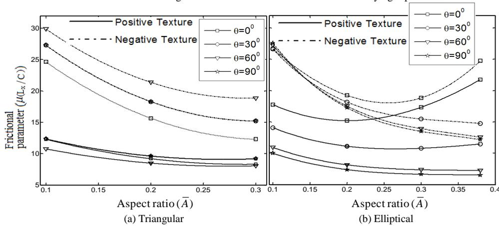
Fig. 9 Effect of orientation on friction parameter with varying aspect ratio
