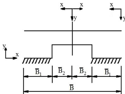
Fig 1. Rayleigh step bearing
