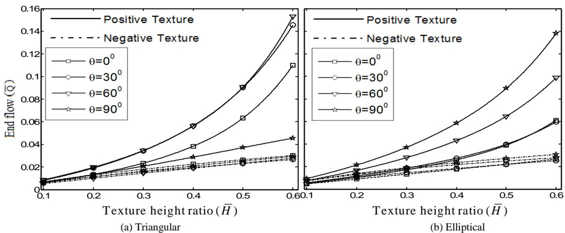
Fig. 5 Effect of orientation on end flow with varying texture height ratio
