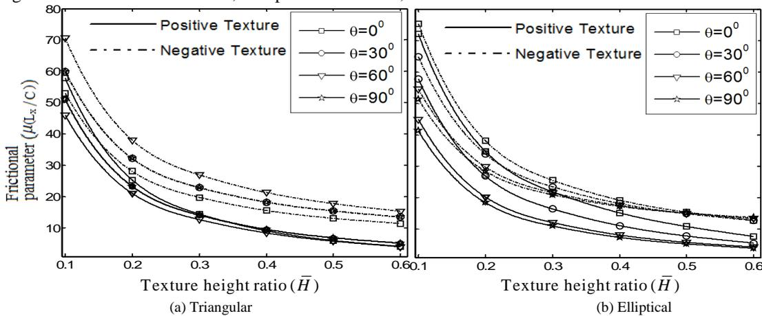
Fig. 6 Effect of orientation on friction parameter with varying texture height ratio
