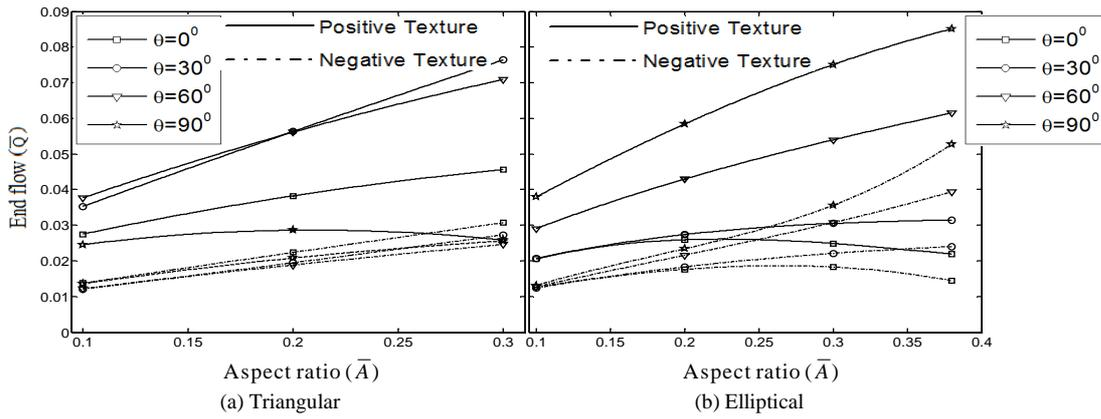
Fig. 8 Effect of orientation on end flow with varying aspect ratio
