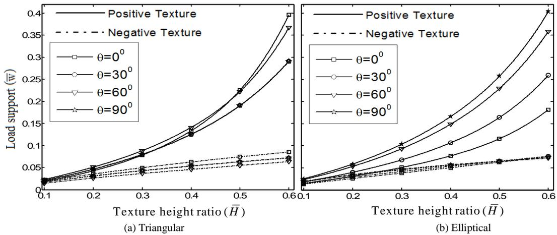
Fig. 4 Effect of orientation on load support with varying texture height ratio
