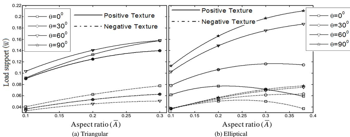
Fig. 7 Effect of orientation on load support with varying aspect ratio
