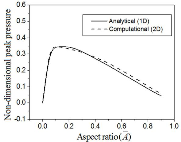
Fig. 2 comparison of the non-dimensional peak pressure
