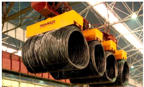
Fig. 4. Coil form Rebars
