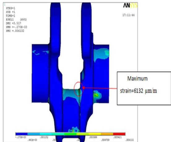
Fig.6.4 Tensile strain in crankshaft
