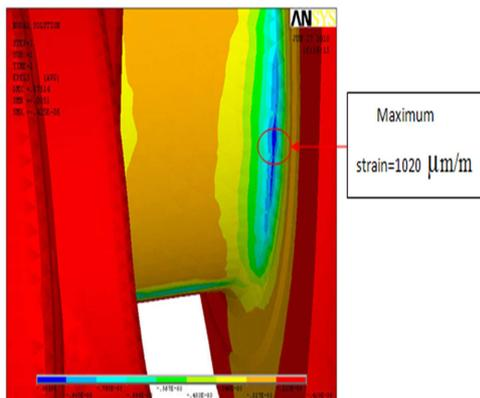
Fig.6.10 Compressive strain in crankshaft
