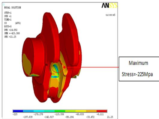
Fig.6.9 Compressive stresses in crankshaft
