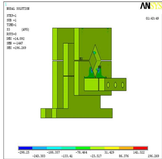
Fig.6.11 Third principle stresses in V-block
