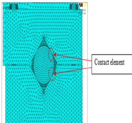
Fig.6.2 Contact element between V-block & crankshaft
