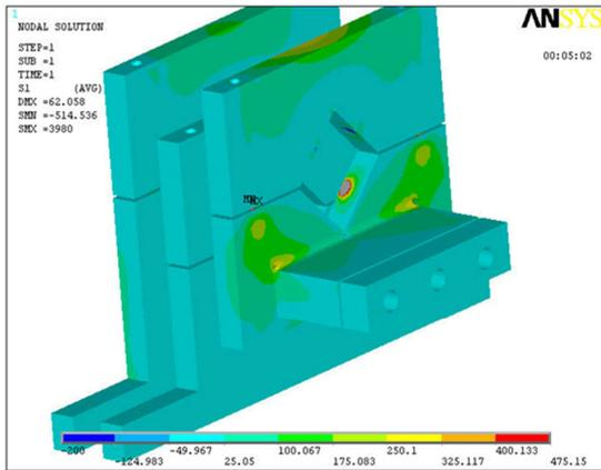
Fig.6.57 First principle stresses in V-block
