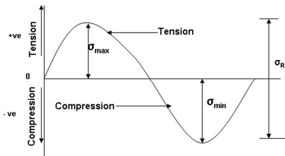
Figure 3.1: Fully reversed load cycle
