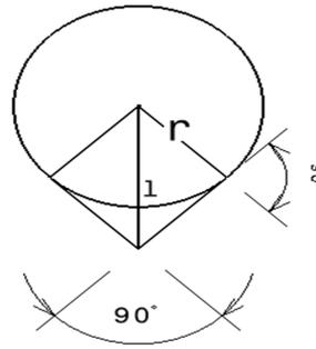
Suppose  $r$  is radius of crank pin or journal which will clamp in v-block then depth of V-block is,
