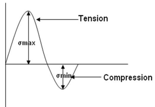
Figure 3.2: Variable load cycle
