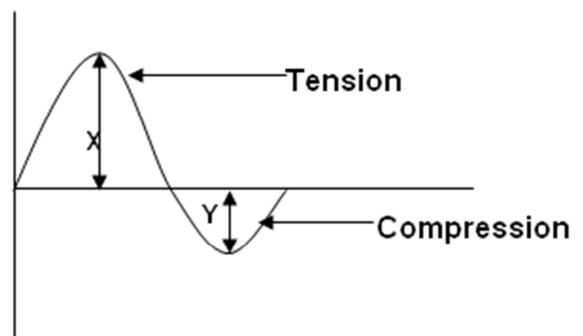
Figure 3.3: Variable load cycle
