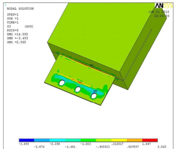
Fig.6.12 Third principle stresses in load transfer plate
