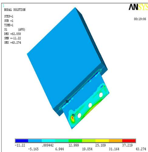
Fig.6.6 First principle stresses in load transfer plate
