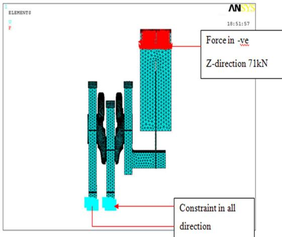
Fig.6.1 Boundary condition For tensile load
