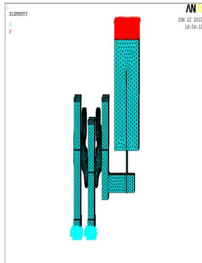
Fig.6.7 Boundary condition for compressive load
