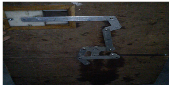
Fig.5. Fabricated model of the switchgear mechanism
