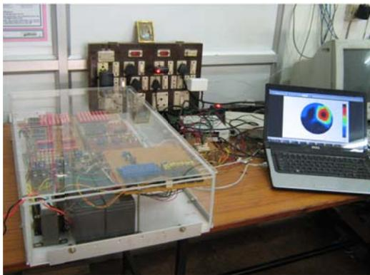
Fig. 3. The complete battery based EIT system.
