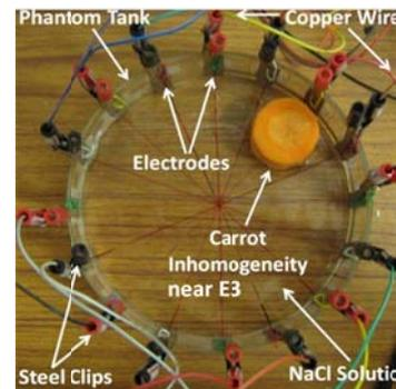
Fig. 4. NaCl-carrot phantom with carrot cylinder near electrode 3 (E3) as the inhomogeneity.
