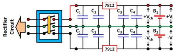
Fig. 2. Schematic of the battery based regulated power supply (BRPS) with filter-regulator-filter (FRF) block.
