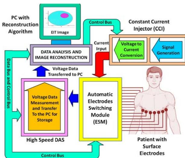
Fig. 1. EIT system schematic with a patient with surface electrodes.
