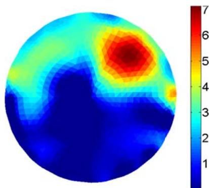
Fig. 5. Resistivity image of the NaCl-carrot phantom (shown in Figure 4) with carrot cylinder near electrode 3 (E3) as the inhomogeneity.
