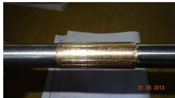
Fig..4. The shaft with a press fitted gun metal sleeve having longitudinal grooves.
