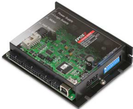
Figure 3 the EPOS 2 is an upgraded positioning controller. Thanks to interpolated position mode (IPM), the EPOS2 is able to synchronously traverse a path set by support points.
