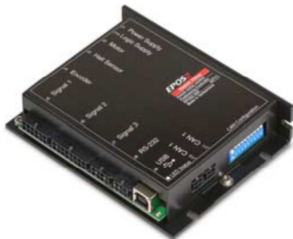
Figure 4 the EPOS2 50/5 (with USB) is tuned to DC brush motors with encoder or brushless EC motors with Hall sensors and encoder, from 5 to 250 watts.
